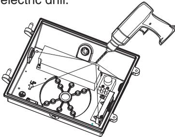
5. Drill a hole in the wall with an electric drill.
