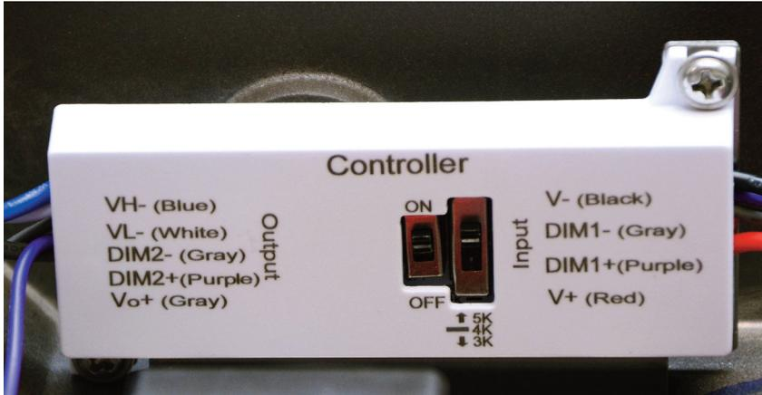
Use on/off switch to control fixture’s photocontrol. Use CCT switch to adjust color temperature. (3000K or 4000K or 5000K.)
