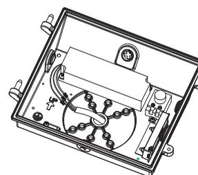
10. Install the cover of the fixture and connect the terminal block.
