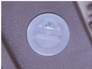
PC is located on a side conduit hole behind the translucent ½” threaded conduit plug. The translucent plug needs to be securely tight for a seal. The plug allows light through so that the PC can respond to dusk and dawn.
