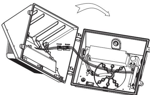
11. Fix the fixture with screws.
